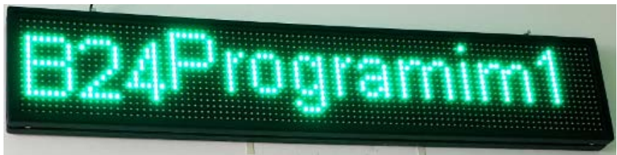
Figure 4. Panel Microcontroller and electronic Card Model HD-E65 for LED Diodes of Panel 96 × 16
