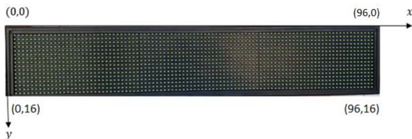
Figure 26. Screen respectively LED display with 96 \times 16 enlightening diodes as well as pixel distribution by axis x and y
